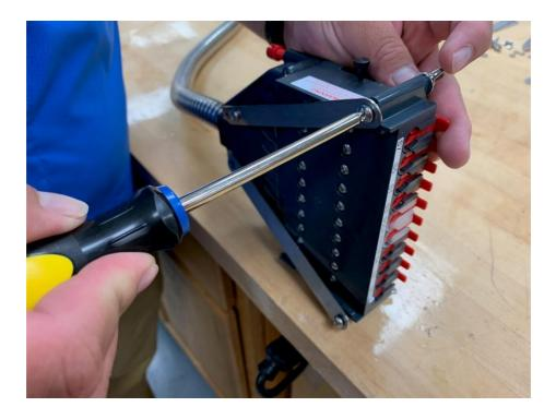
Use a Phillips screwdriver to tighten the wing nut. The wing nut should be finger tight, the stainless bracket will bow slightly as shown below.
